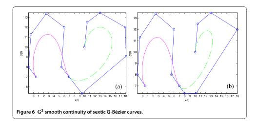
$\gamma$  = 2/3 in Figure 6(a), and  $\alpha$  = 3/2 and  $\gamma$  = 3/4 in Figure 6(b). The broken lines and circular points in Figure 6 indicate the same features as in Figure 2. Figure 6 shows that the second and third control points of the second curve in the splicing curves are altered by changing the value of two scale factors, thus changing the shape of the second curve.
