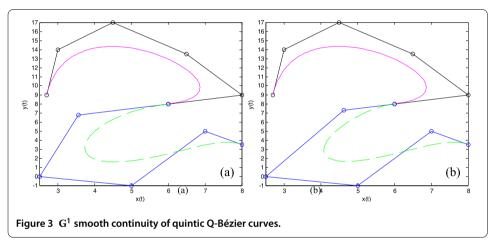
(1,2,-1,1), respectively, as well as a scale factor of  $\alpha=1$ . The second example is a quartic Q-Bézier curve spliced with a quintic Q-Bézier curve, where the shape parameters are  $(\lambda_1,\lambda_2,\lambda_3,\lambda_4,\lambda_5)=(-4,-1,1,2,1)$  for the quintic Q-Bézier curve, with a scale factor of  $\alpha=7/2$ . The broken lines indicate the control polygons of the Q-Bézier curves; the circular points indicate control points for the curve.
