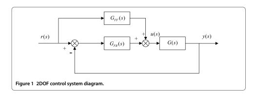
The transfer function of the entire 2DOF control system  $G_{2DOF}(s)$  from the reference signal r(s) to actual outputs y(s), is given by
